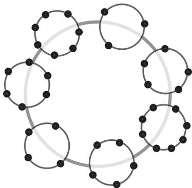
**Fig. 1.** The global topology of Herbivore is structured as a ring, with each clique assigned a unique key. While communication in Herbivore is primarily done at the clique level, nodes can leverage this global backbone to communicate with other cliques
