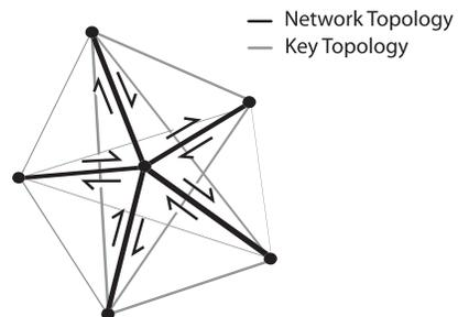
**Fig. 3.** A Six Node Clique. While the network topology is star-shaped to ensure high bandwidth utilization and low latency, the key topology is a complete graph to protect anonymity. Since the center of the star has a disproportionate network load, Herbivore selects a new center for each round by cycling through the clique members.
