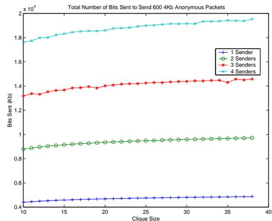
**Fig. 8.** Number of bits sent to transmit a constant amount of data.
