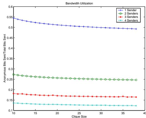
**Fig. 7.** Effective bandwidth utilization ratio for varying numbers of simultaneously active senders.
