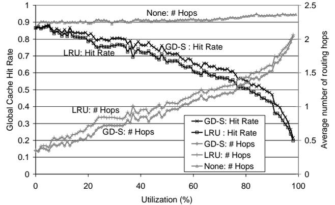
**Figure 8: Global cache hit ratio and average number of message hops versus utilization using Least-Recently-Used (LRU), GreedyDual-Size (GD-S), and no caching, with  $t_{pri} = 0.1$  and  $t_{div} = 0.05$ .**
