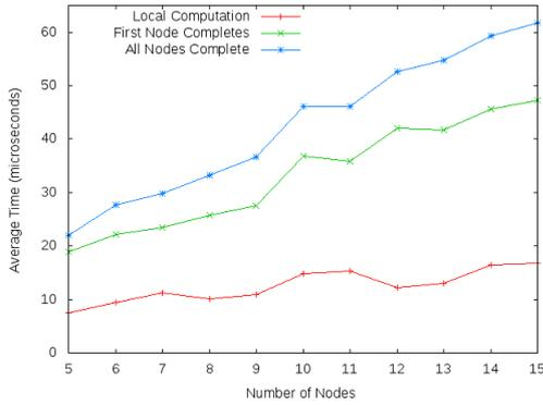
**Figure 13: Time for nodes to install new routing tables after a link change**
