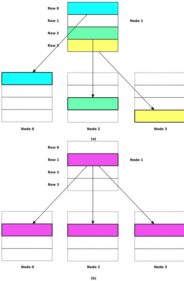
**Figure 2: Illustration of SST-reads vs SST-writes. Node  $i$  owns row  $i$  of the table for  $i = 0,1,2,3$ . In (a), Node 1 reads the rows 0,2,3 from their respective owners. In (b), Node 1 writes its local row at all the nodes.**
