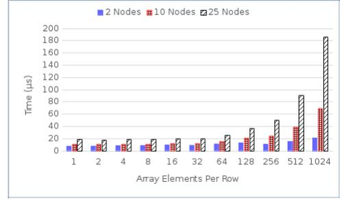
**Figure 10: Latency of predicate detection with number of nodes for different number of row elements**
