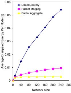
Figure 5: Average Dissipated Energy vs. Network Size
