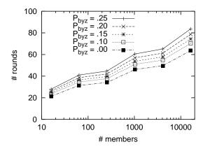
Figure 5: The maximum of 100 simulation experiments of the number of rounds required to disseminate an update to all correct members as a function of the total number of live members for various  $P_{byz}$ . In these experiments,  $\varphi = .99999$ .
