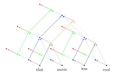
Figure 2: Operation of a 3-layer **deep recursive neural network**. Red and black points denote output and input vectors, respectively; other colors denote intermediate memory representations. Connections denoted by the same color-style combination are shared (i.e. share the same set of weights).
