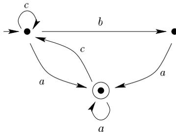
accepts those words over the alphabet  $A = \{a, b, c\}$  where no  $a$  is succeeded by a  $b$ , any  $b$  is succeeded by  $a$ , and  $a$  is the last letter. These three conditions can be expressed by a first-order formula, using variables  $x, y, \dots$  for letter positions,
