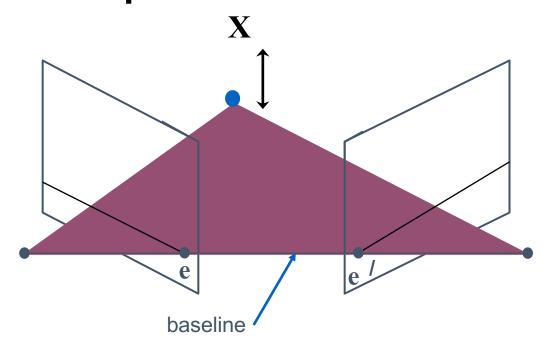
As the position of the 3D point X varies, the epipolar planes "rotate" about the baseline. This family of planes is known as an epipolar pencil (a pencil is a one parameter family).
