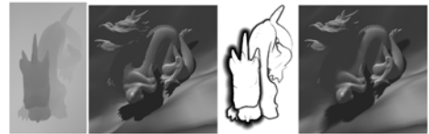
Figure 8: Using a standard shadow map results in hard shadows (left), add a penumbra map to get soft shadows (right). Using a 10k polygon dragon model for the shadows and a 50k polygon model to render, we get 14.3 fps at 1024x1024.
