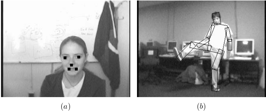
Figure 1: Detection results for a face (a); and a human body (b). Each image shows the globally best location for the corresponding object, as computed by our algorithms. The object models were learned from training examples.
