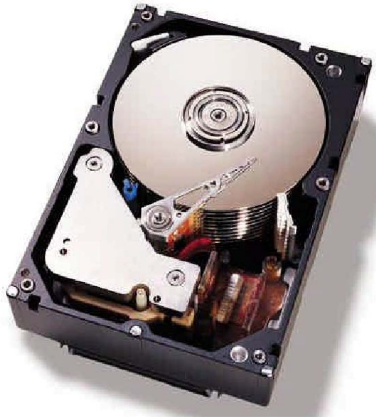
Top view of a 36 GB, 10,000 RPM, IBM SCSI server hard disk, with its top cover removed. Note the height of the drive and the 10 stacked platters. (The IBM Ultrastar 36ZX.)
