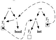
The solution proceeds by first splitting the equation into two equations  $T_1 = T_3 + \text{int}$  and  $T_1 * \text{bool} = T_2$ . The first of these is solved by making  $T_1$  point to the + node. The second is solved by making  $T_2$  point to the \* node. We never need to set the cell for the  $T_3$  node. Notice that we only have to do constant work to solve  $T_1$ , because updating its pointer once effectively substitutes it throughout all the equations.
