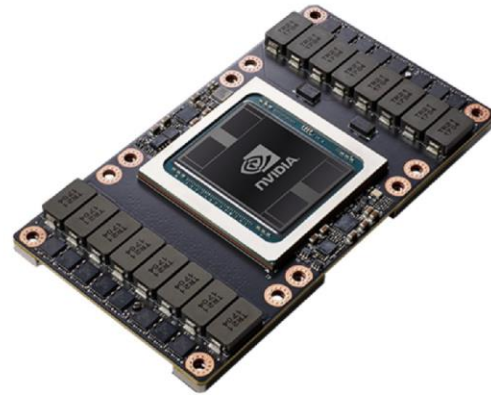
NVIDIA Tesla V100 = 125 TFLOPs of compute
