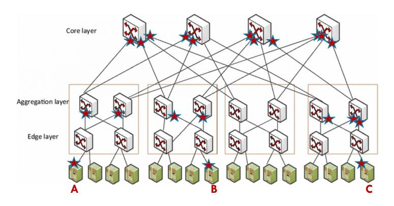
★ means: If you receive a message to address x (on any incoming link), forward it via this outgoing link
