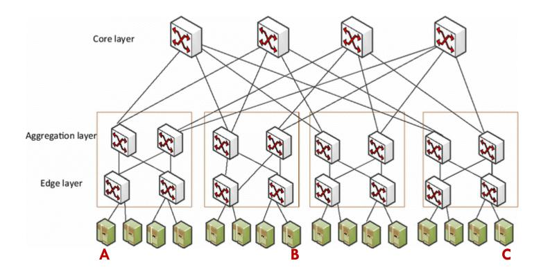
So-called FAT tree topology has at least 2 routes between each pair of nodes for fault-tolerance
