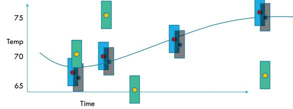
Then we wanted to combine the output by looking for a "box overlap" to compensate for sensor errors.
