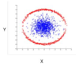
Any form of linear projection method to one dimension on this data will merge the red and blue points together thus losing information about the original dataset. This is because one needs to consider non-linear projection to one dimension to obtain separation of red and blue points.
