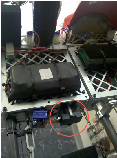
Fig. 2. The Inertial Measurement Unit (IMU, circled in red) is used to estimate the ground slope.
