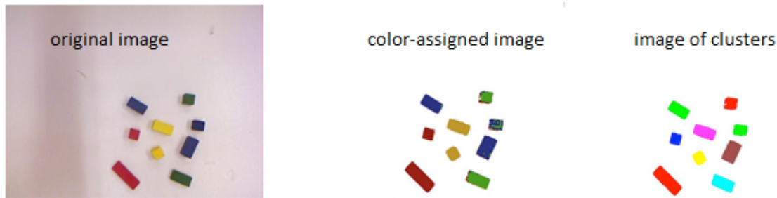
Figure 2: (left) The original image taken by the Kinect camera. (middle) The image created by reassigning RGB values to each pixel depending on whatever color classification the RGB values of each pixel most closely resembles. For example, pixels with RGB values most closely resembling red are assigned a value of pure red. (right) This image represents which pixels belong to which cluster. The red pixels all belong to the cluster #1; the green pixels all belong to cluster #2 and so on
