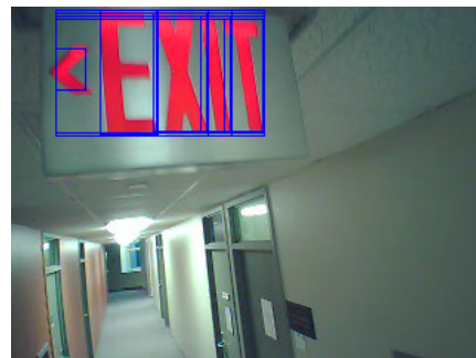
Figure 2: All the bounding boxes whose features are fed into the SVM. There are 15 in this image.
