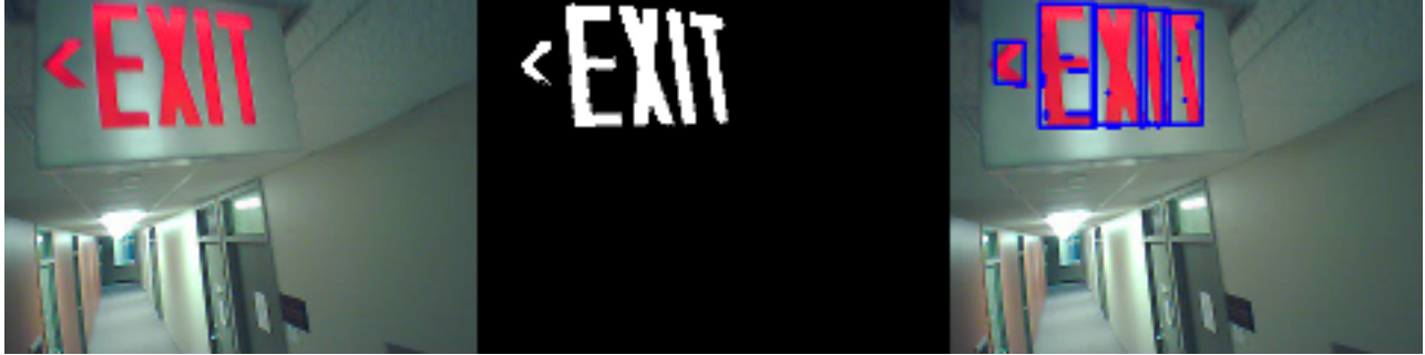
Figure 1: Stages in the image processing. From left to right: initial image, thresholded image, bounding boxes
