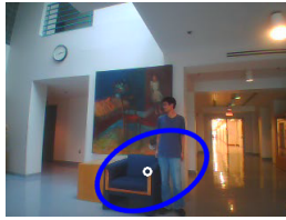
Fig. 2. Camshift on a distracting background. It was initialized to track the blue shirt, but eventually tracked the blue chair instead. The Kalman filter dynamically penalizes CamShift with a higher variance.
