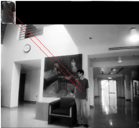
Fig. 3. SURF on the same distracting background as Fig. 2. SURF successfully follows two points on the shirt from one frame (top) to the next (bottom); the red lines link these points across the frames.
