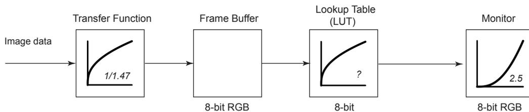
Before the image is stored in the framebuffer, it goes through a transfer function so that it is stored in the framebuffer with a nonlinear quantization at gamma 1.47. The framebuffer uses an 8 bit integer format. The graphics hardware has to convert the format of the framebuffer to the display's pixel format. This is done using a simple lookup table (LUT).
