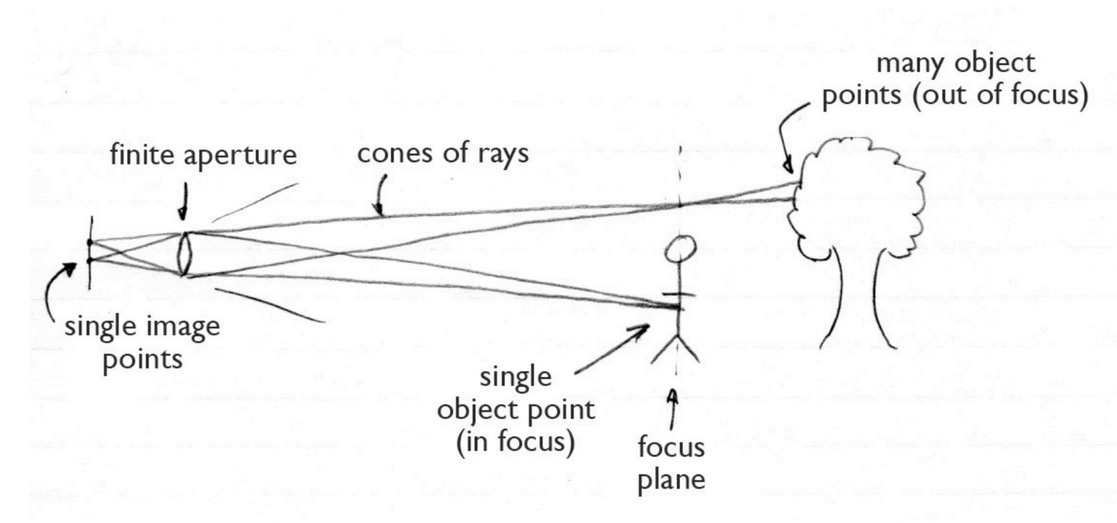
finite aperture produces limited depth of field
