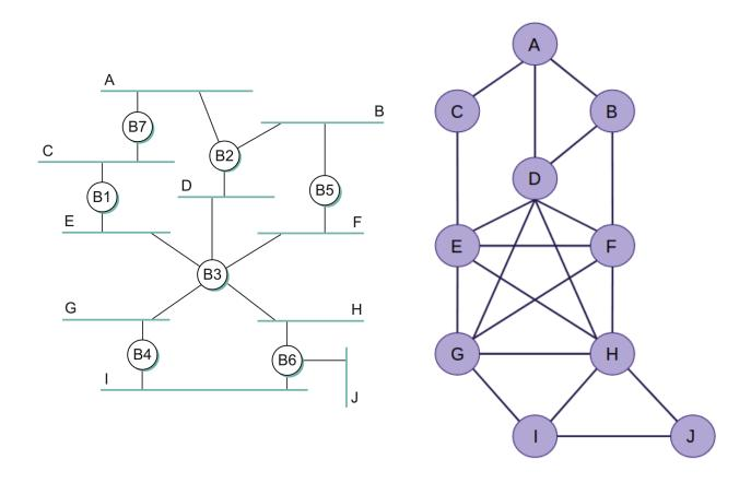
Above an extended LAN and its corresponding network graph is given.
