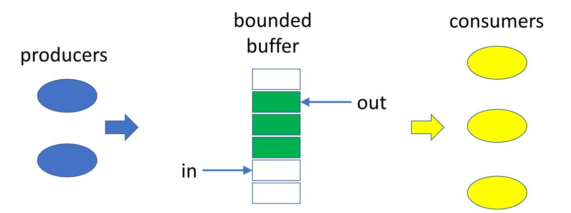
Producers block when buffer is full Consumers block when buffer is empty
