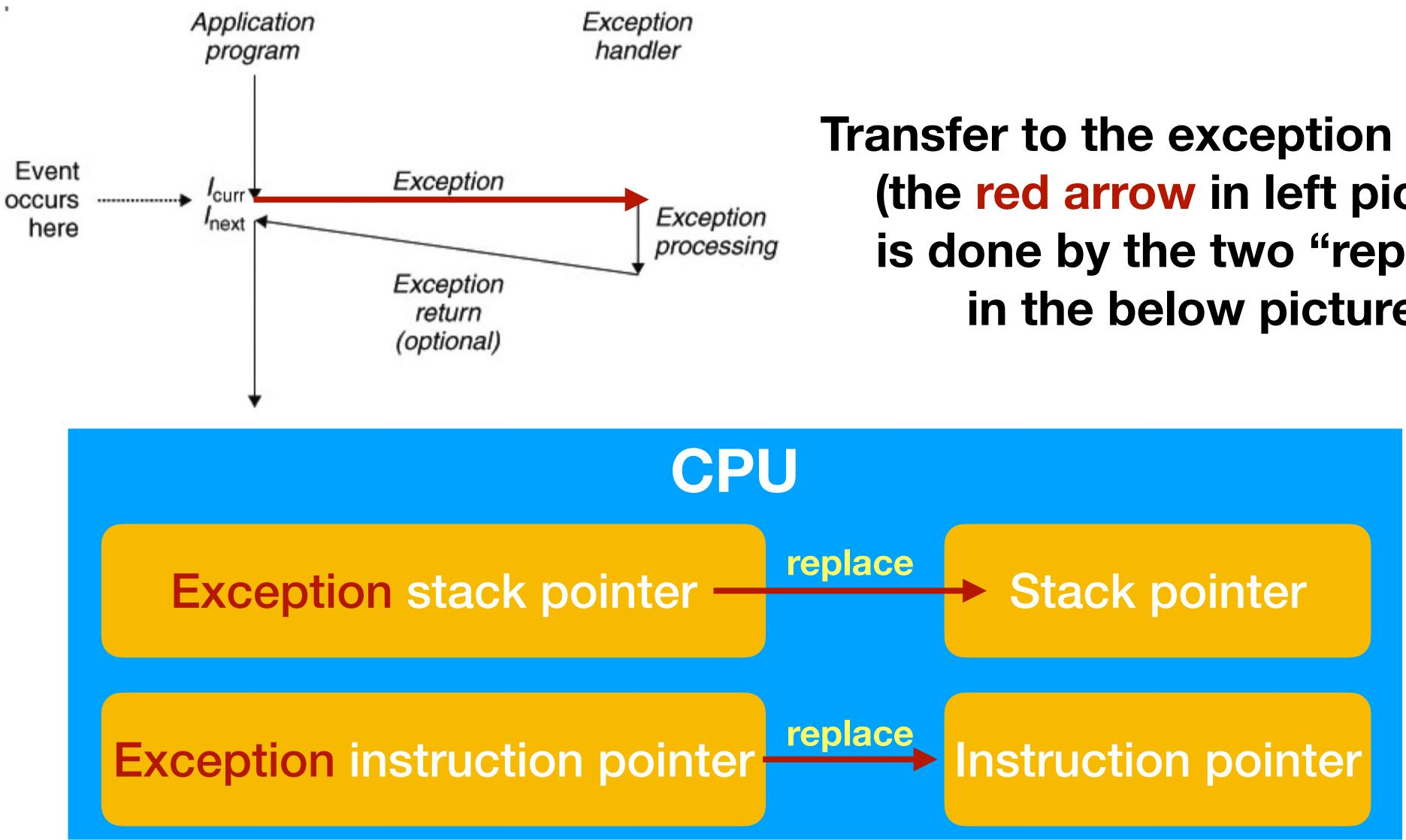
**Transfer to the exception handler** (the red arrow in left picture) is done by the two "replace" in the below picture.
