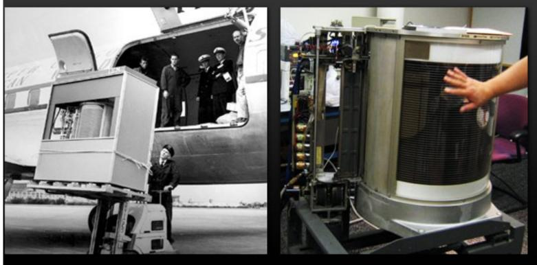
The first hard disk drive—the IBM Model 350 Disk File (came w/IBM 305 RAMAC, 1956).
