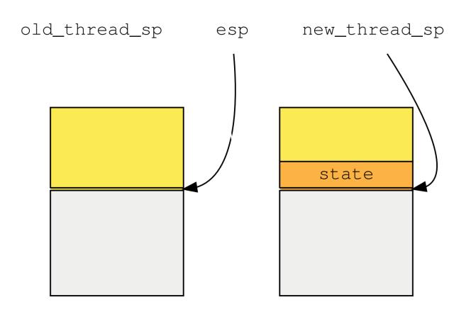
The stack pointer still points to the old thread's stack, while the new thread is stored somewhere else in memory.
