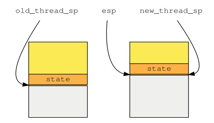
Now we can move the stack pointer to the new thread's stack now.
