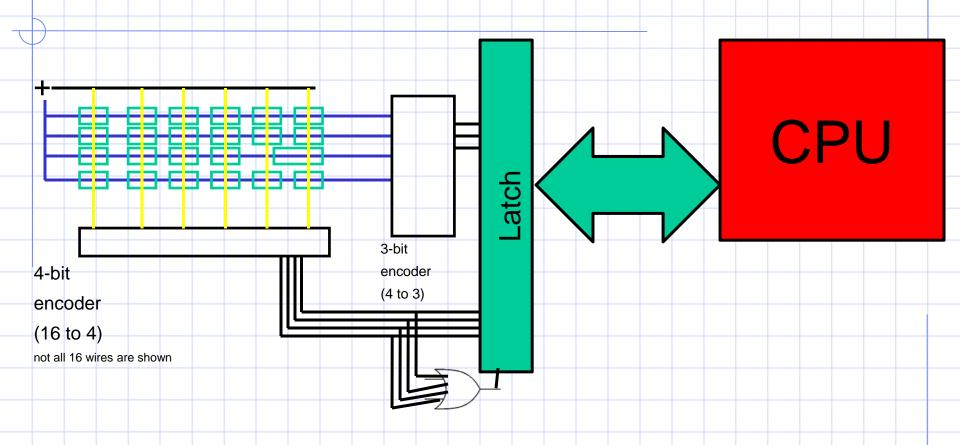
The keyboard can then appear to the CPU as if it is a special memory address
