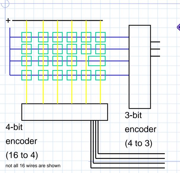
When a key is pressed, a 7-bit key identifier is computed
