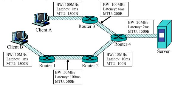
The above figure illustrates a network in which two clients (Client A and Client B) route packets through the network to the server. Each link is characterized by its Bandwidth (BW), one-way Latency, and Maximum Transfer Unit (MTU). All links are full-duplex (can handle traffic in both directions at full bandwidth).
