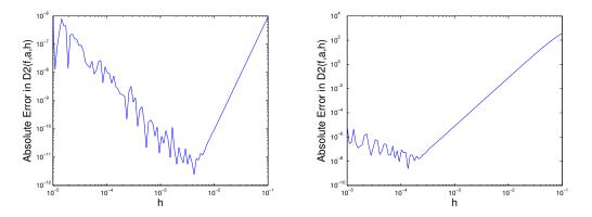
The total error that is displayed in these plots is a combination of roundoff error and "math error". Model the total error as a function of h and use it to explain the shape of the graphs and what determines the best value of h. Notice that the optimum h values and the minimum error values are rather different in the two examples. Offer a possible explanation. Be brief! No proofs necessary.
