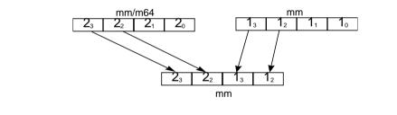
Code in the <u>Example 4-6</u> unpacks two packed-word sources in a non-interleaved way. The goal is to use the instruction which unpacks doublewords to a quadword, instead of using the instruction which unpacks words to doublewords.
