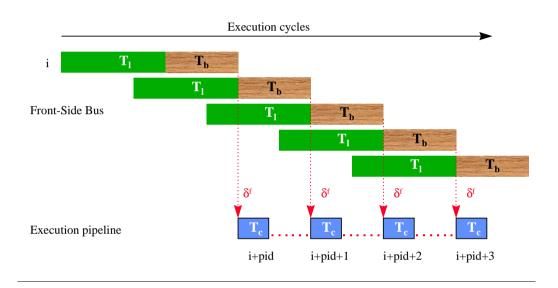
The following relationship calculates the prefetch scheduling distance (or prefetch iteration distance) for the case when memory throughput latency is greater than the compute latency.
