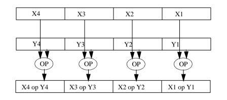
SIMD computations like those shown in Figure 1-1 were introduced into the IA-32 architecture with the MMX<sup>TM</sup> technology. The MMX technology allows SIMD computations to be performed on packed byte, word, and doubleword integers that are contained in a set of eight 64-bit registers called MMX registers (see Figure 1-2).
