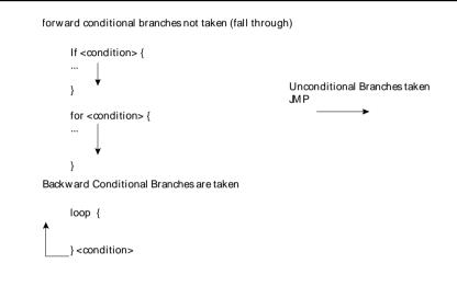
Examples <u>2-6</u>, <u>2-7</u> provide basic rules for the static prediction algorithm.
