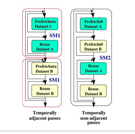
For Pentium 4 processors, the left scenario shows a graphical implementation of using prefetchnta to prefetch data into selected ways of the second-level cache *only* (SM1 denotes strip mine one way of second-level), minimizing second-level cache pollution. Use prefetchnta if the data is only touched once during the entire execution pass in
