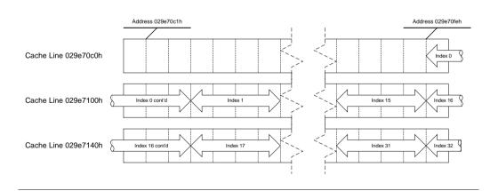
Alignment of code is much less of an issue for the Pentium 4 processor than for earlier processors. Alignment of branch targets to maximize bandwidth of fetching cached instructions is an issue only when not executing out of the trace cache.
