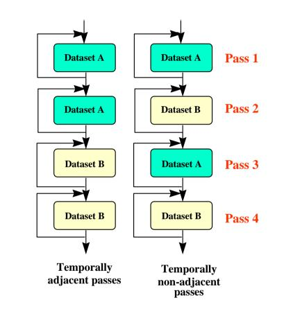
In the temporally-adjacent scenario, subsequent passes use the same data and find it already in second-level cache. Prefetch issues aside, this is the preferred situation. In the temporally non-adjacent scenario, data used in pass m is displaced by pass (m+1), requiring data re-fetch into the first level cache and perhaps the second level cache if a later pass reuses the data. If both data sets fit into the second-level cache, load operations in passes 3 and 4 become less expensive.
