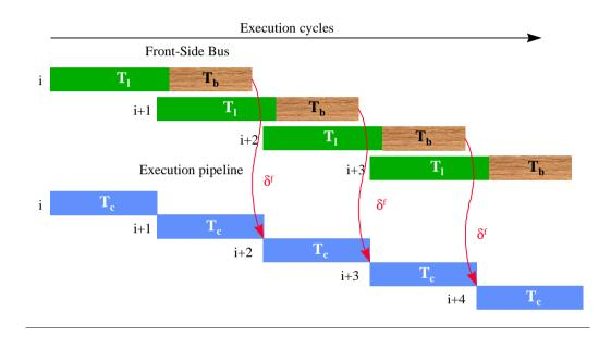
For this particular example the prefetch scheduling distance is greater than 1. Data being prefetched for iteration *i* will be consumed in iteration i+2. Figure 6-12 represents the case when the leadoff latency plus data transfer latency is
