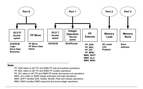
**Port 0**. In the first half of the cycle, port 0 can dispatch either one floating-point move  $\mu$ op (including floating-point stack move, floating-point exchange or floating-point store data), or one arithmetic logical unit (ALU)  $\mu$ op (including arithmetic, logic or store data). In the second half of the cycle, it can dispatch one similar ALU  $\mu$ op.
