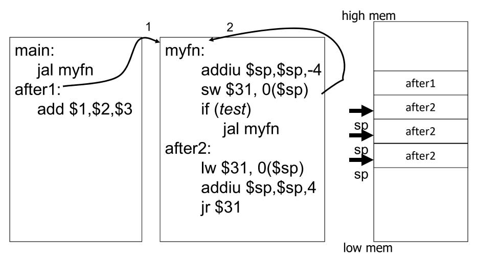
Stack used to save and restore contents of \$31
