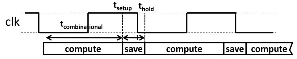
Edge-Triggered  $\rightarrow$  signals must be stable near falling edge "near" = before and after  $t_{setup} \qquad t_{hold}$
