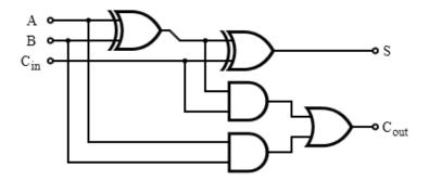
In the above diagram, A and B are the 1-bit inputs, while  $C_{in}$  is the carry-in bit. S is the output bit, while  $C_{out}$  bit is the carry-out bit. This is the optimal circuit for the following truth table:
