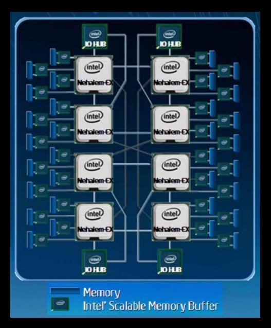
8 multiprocessors4 core per multiprocessor2 HT per core
