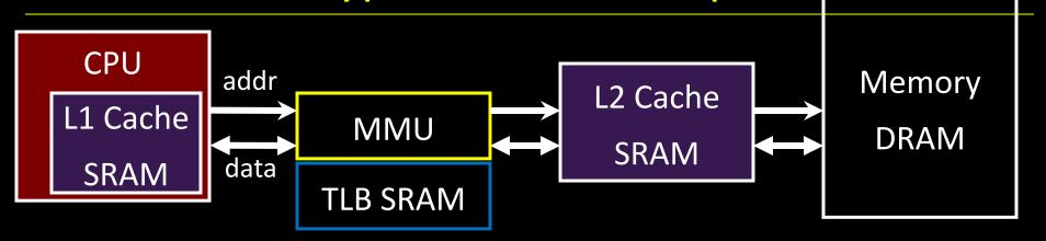
Typical L1: On-chip virtually addressed, physically tagged
