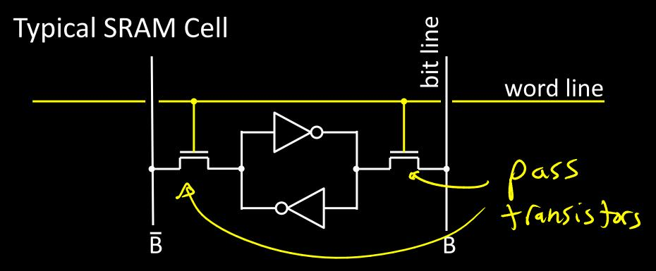
Each cell stores one bit, and requires 4 – 8 transistors (6 is typical)
