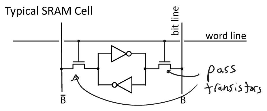
Each cell stores one bit, and requires 4 – 8 transistors (6 is typical) Read:
