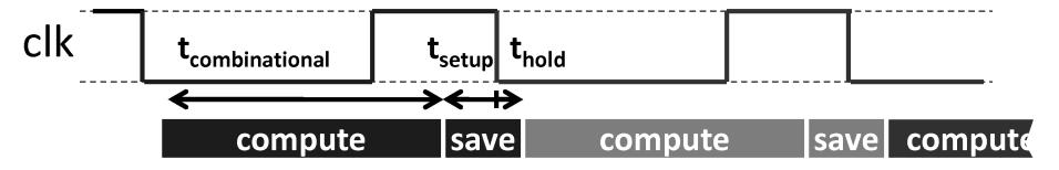
Signals must be stable near falling clock edge
