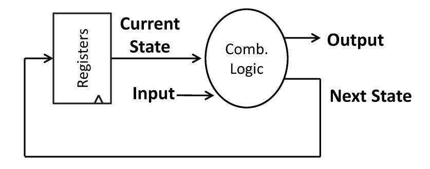
Outputs and next state depend on both current state and input
