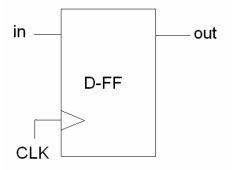
On a positive edge of the clock signal, the D Flip-flop passes the input value to the output.
