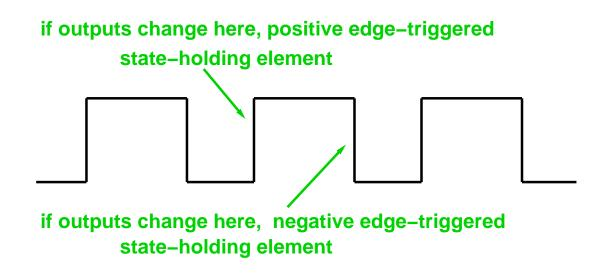
• Inputs must be stable just before the clock edge where the outputs change.
