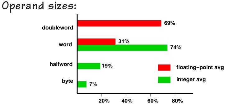
$\Rightarrow$  support 8-bit, 16-bit, 32-bit integer, and 32-bit and 64-bit floating-point.
