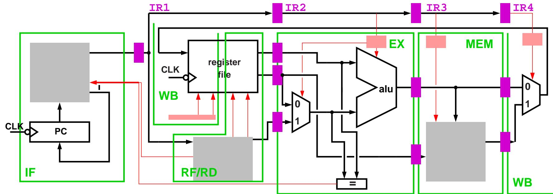
Basic idea: copy the instruction, and generate local control in each pipeline stage.
