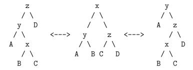
See <u>this page</u> for a nice visualization of splay tree rotations and a demonstration that these rotations tend to make the tree more balanced while also moving frequently accessed elements to the top of the tree.
