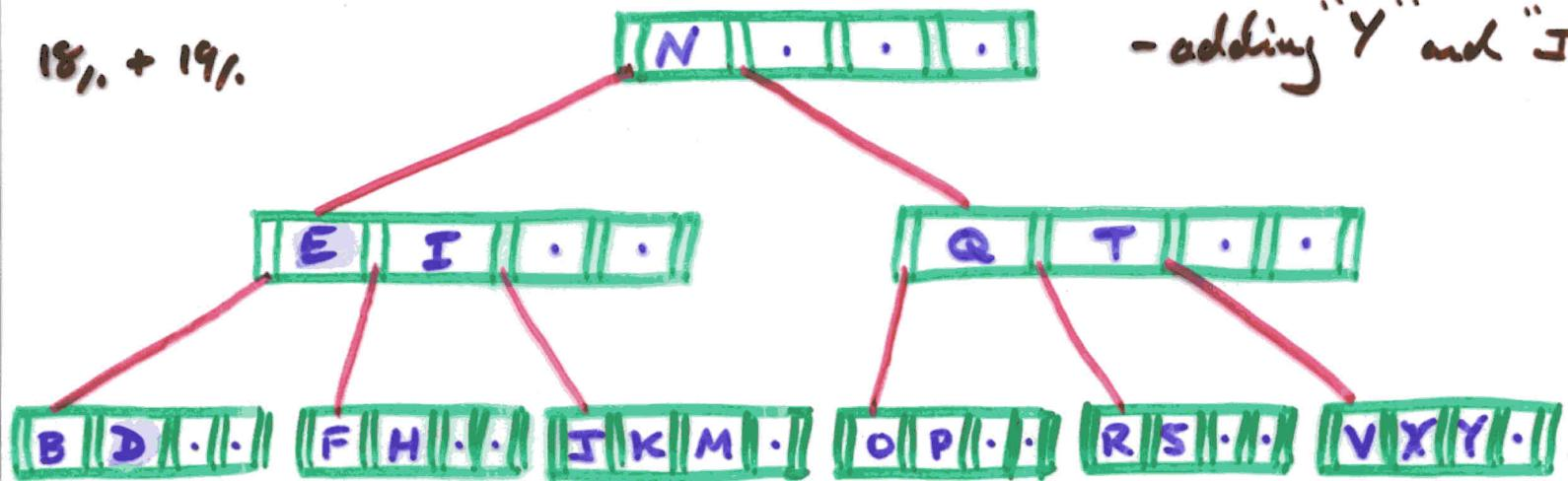
Note that each addition is passed all the way down to a leaf — the non-leaf nodes are only created as needed to hold medians of overflows.
