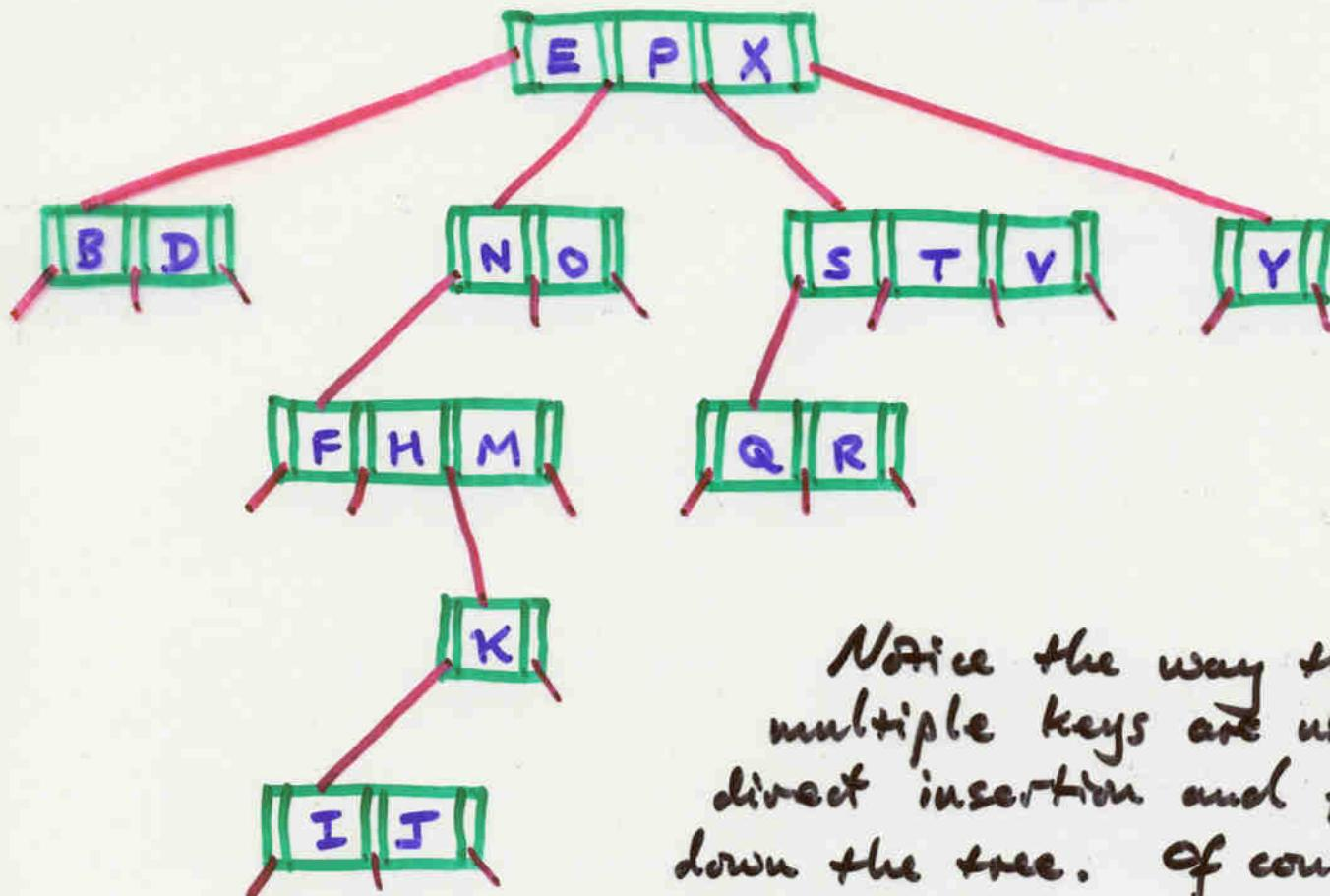
Notice the way that multiple keys are used to direct insertion and find down the tree. Of course, this structure raises the same questions about balance as we saw with the 2-way (binary) search trees.
