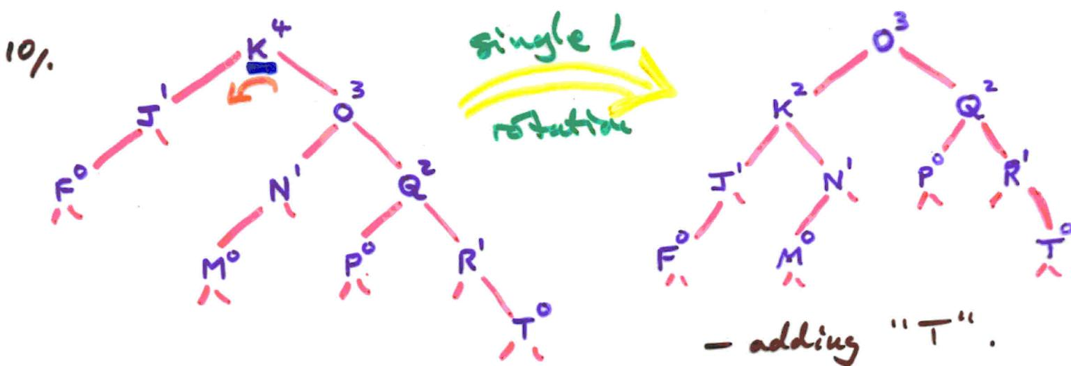
At each stage we underlined (in blue) the 'lowest' node which had excessively unbalanced subtrees. The natural question is how do decide whether to expect to do a single or double rotation. The effective answer is to perform a single rotation if the additional length is to the outside of the child of the affected node, and to perform a double rotation if it's to the inside of that child.
