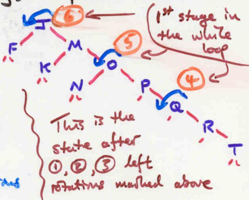
Notice that it's quite important to do the first few left rotations before embarking on the while loop. Also, it's important to work backwards once the rotation pivots have been selected, if we're to finish with a perfectly balanced tree (or at least as well-balanced as possible).
