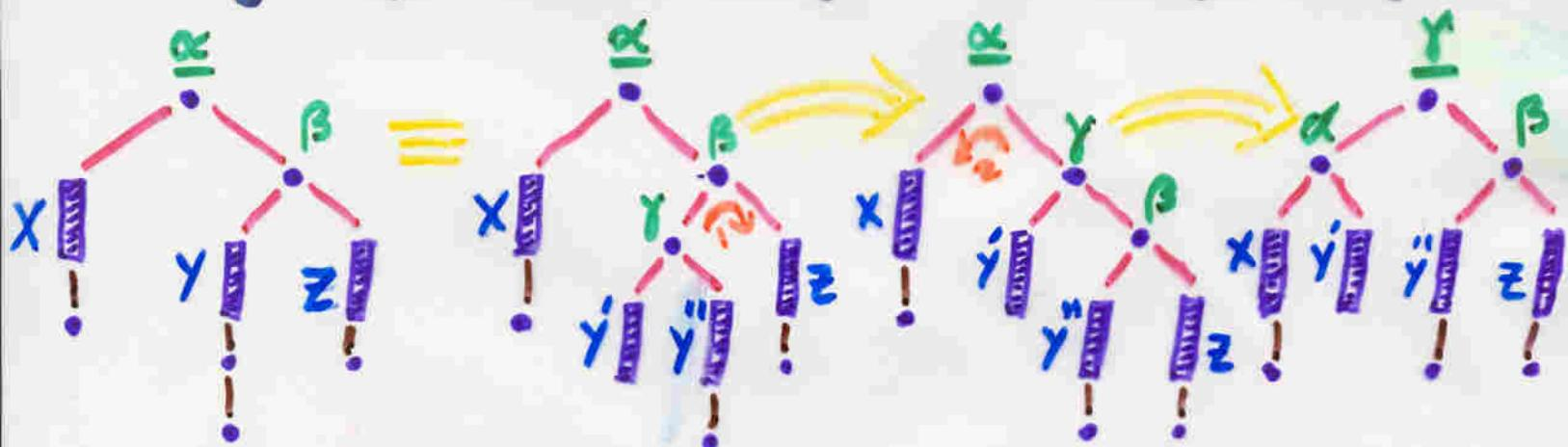
It doesn't matter whether  $Y'$  or  $Y''$  is regarded as longer (they could both be equally long). So a double left rotation is really a single right rotation at the child level followed by a single left rotation at the parent level. Thus step 5<sub>1</sub> becomes ...
