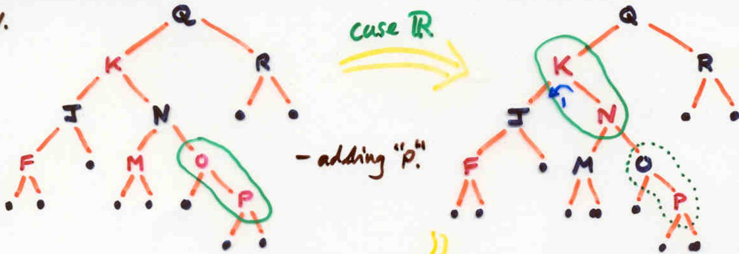
Notice that this is an example of the re-colouring causing the problem to propagate up the tree.
