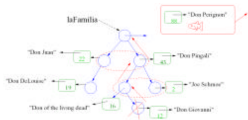
Heapifying after removing root element
