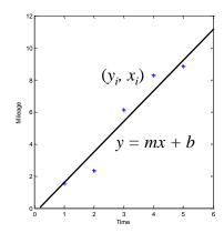
The line won't necessarily pass through any data point
