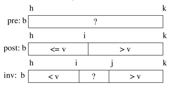
Called binary search because each iteration of the loop cuts the array segment still to be processed in half
