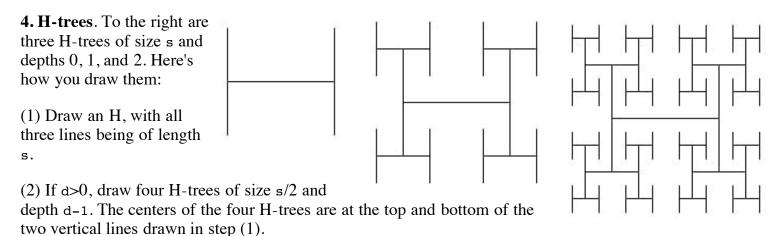
H-trees are useful in designing microprocessor chips. The lines are wires that connect circuit components in a tree of interconnections, witout wires crossing.
