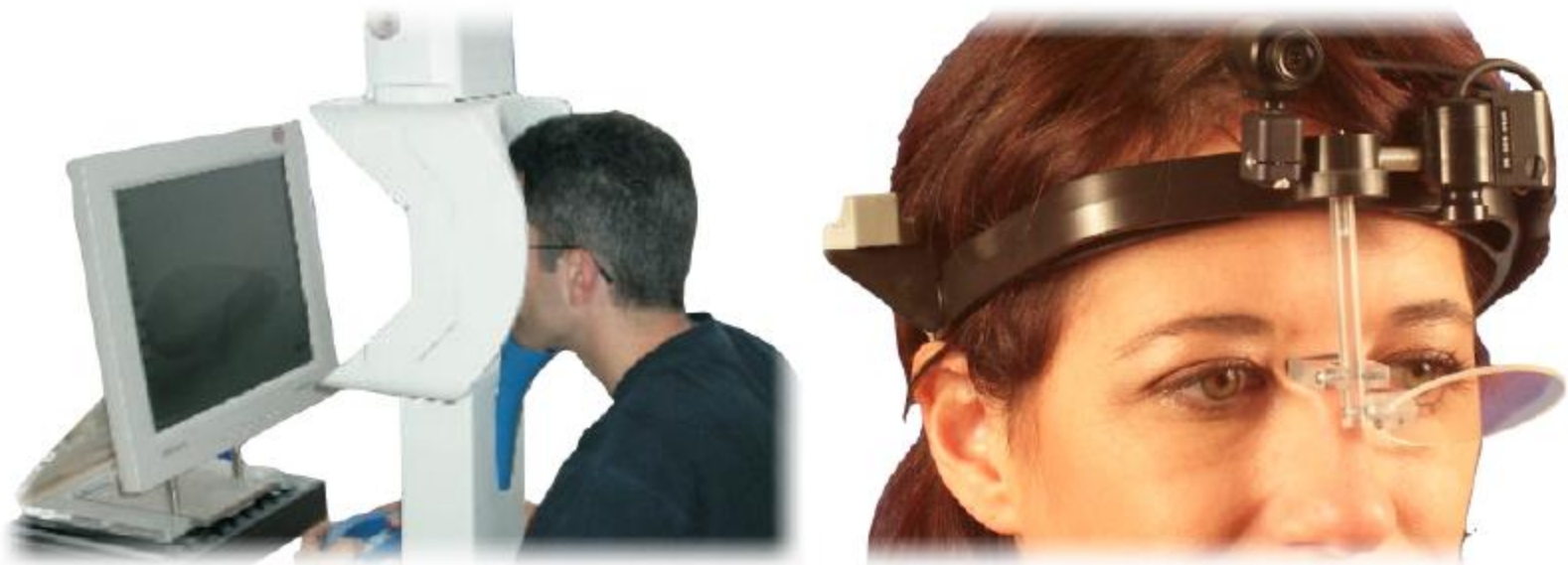
Figure 2.2: Typical eye trackers used for cognitive pupillometry. The eye tracker on the left is an SMI iView X chin-rest style instrument, used primarily for reading and other high-precision applications [108]. The eye tracker on the right is the Polhemus VisionTrak Standard Head Mounted Eye Tracking System [93], used for mobile applications, especially driving and piloting.
